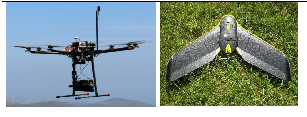
Fig. 4 Octocopter with a light detection and ranging (LiDAR) sensor (left) and fixed-wing eBee drone (right)
