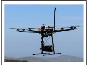
fig. 1 - Oben's octocopter carrying the LIDAR
