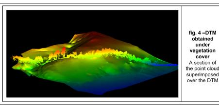
obtained under vegetation cover A section of the point cloud superimposed
